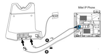
Desk phone connection via USB port or headset port Connect the cables as illustrated.
